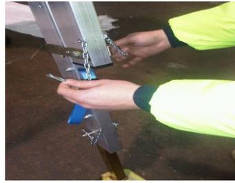
Adjust the height by removing the two Leg Pins and rolling the Mono-Dec Platform up the wall to the desired height and replace both Leg Pins remembering to also replace the safety 'R' Clips provided. After adjusting to height it will be necessary to re-level the Mono-Dec platform by moving the feet either away or towards the wall.
