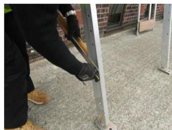
When fitting the Brace the back Leg Foot should be as close to the wall as possible, without fouling the wall or touching the ground. Fit the Pin and 'R' Clip.
