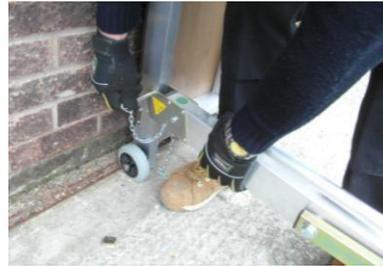
Fit both Legs using the Pins and 'R' Clips provided and ensure that the Pins are inserted outside in, to minimise the risk of the 'R' Clips being Knocked out. **REMEMBER:** Fit the Legs to the 'Normal use' hole Labelled on the underside of the platform.
