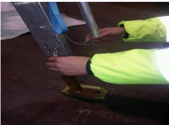
The Feet maybe adjusted in 25mm increments but in extreme cases either Leg can be adjusted Independently. Fit Pins and 'R' Clips to secure.
