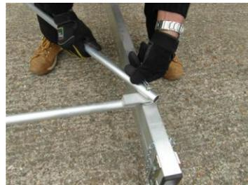
Swing out each brace over to the opposite Leg and secure onto the retaining stud using the two 'R' Clips provided in a downward position.
