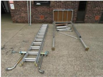
Lay out the components ready for assembly with the platform against the wall with wheels on the ground. Identify the corresponding leg for each side of the platform (Green - Left / Red - Right)
