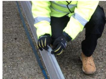
Pull out the 'R' Clips and release the two Braces from their stowed position.
