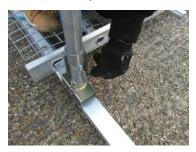
Insert the upright into the Batten socket and secure with the pin and 'R' Clip supplied.
