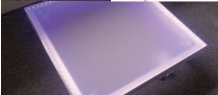
RGB LED touch sensitive perspex platform
