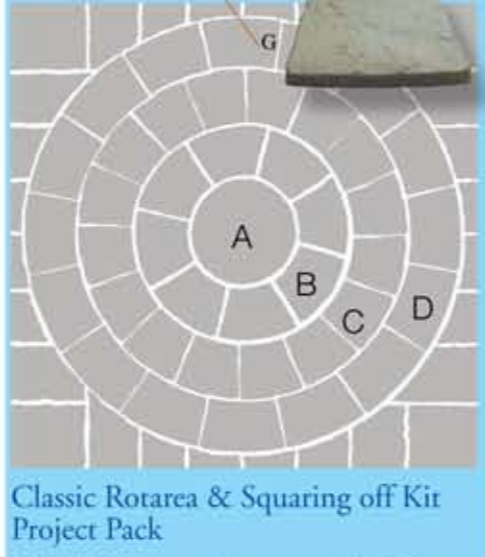
Classic Rotarea & Squaring off Kit Project Pack 3.66m (12') diameter circle squared off to 3.96m sq coverage 15.68 sq m - 69 pieces - 1452kg
