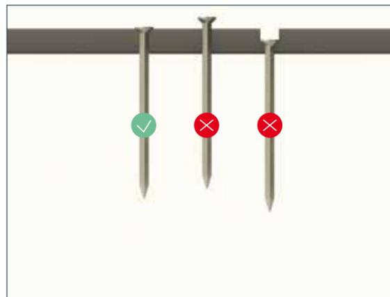
Do not countersink or angle fixings. Surely fixings must not be proud the surface of the plank.
