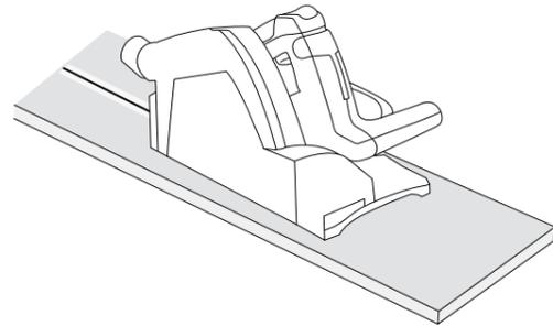
For a non-ventilated and dust free environment, we recommend using Cembrit Mechanical Shear.
