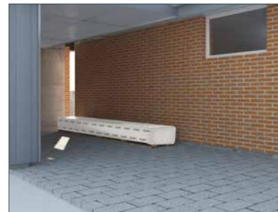
If storing on site for more than 2-3 weeks, the product should be kept under a roof. A maximum of 4 panel or 8 plank pallets can be stored on top of each other.
