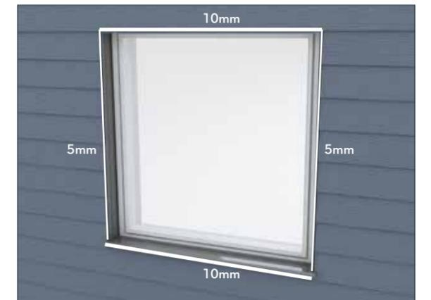
There must be a minimum of 5mm (vertical) and 10mm (horizontal) clearance around windows/ doors-/framing/metal trim and other building materials to allow for structural movements and proper water drainage and ventilation.
