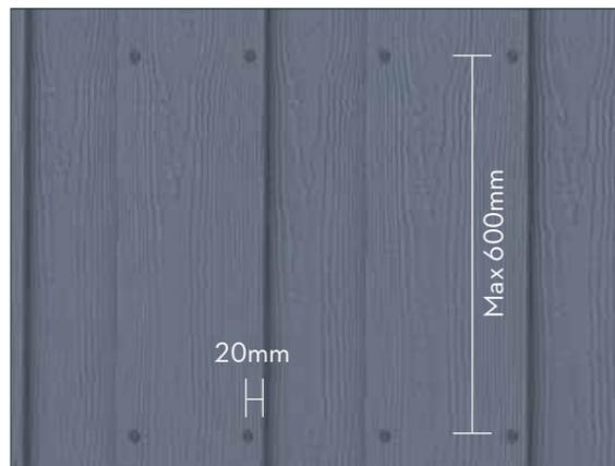
For visible fastening on timber battens, we recommend using Cembril Facade Screw.
