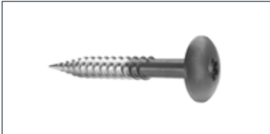
Cembrit Facade Screw wood Without washer SCR-W 4.5x40mm A4 stainless steel (Cembrit Patina)
