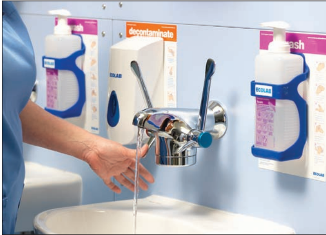
To aid hygienic handwash, the Optitherm's double lever operation allows the tap to be operated using the thumb, then turned off using the elbow or upper forearm, while the outer surface is continuous and smooth for easy cleaning.
