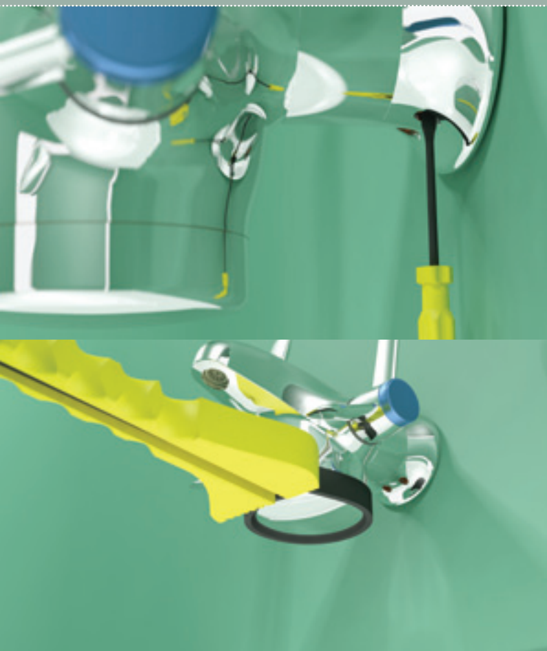
Isolation valves are accessed under the tap spigot
