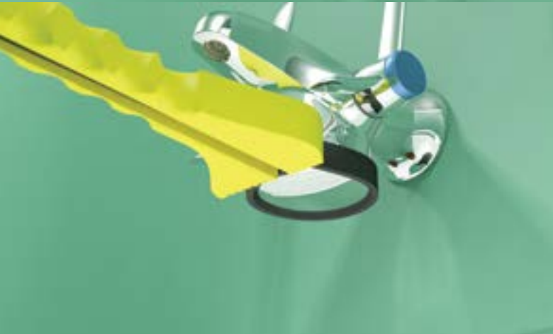
Isolation valves are accessed under the tap spigot
