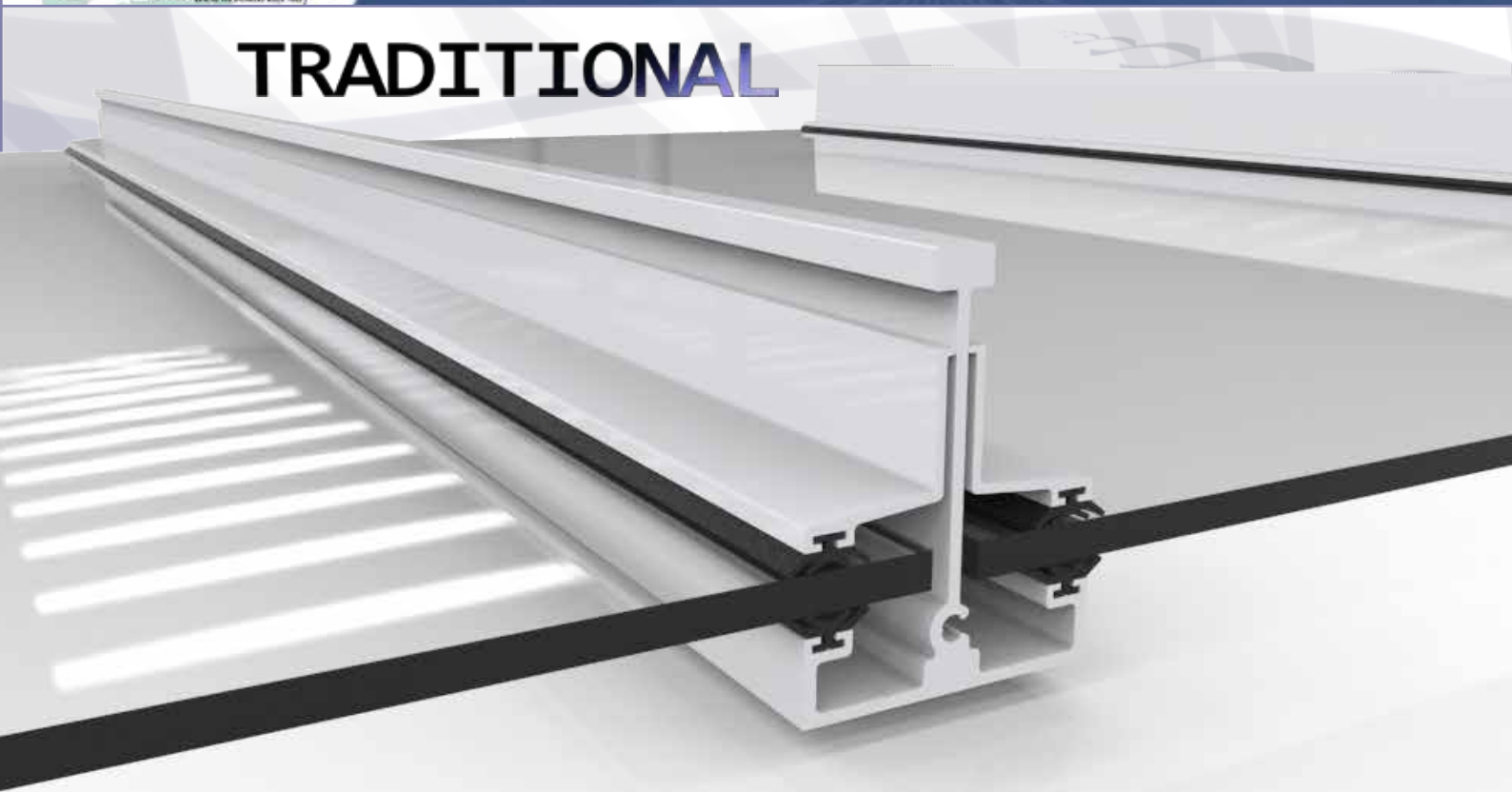
Traditional TW1 type extruded aluminium Glazing Bar with screw-on WT1 wing sections - single glazed with 6-30mm glazed infills.
