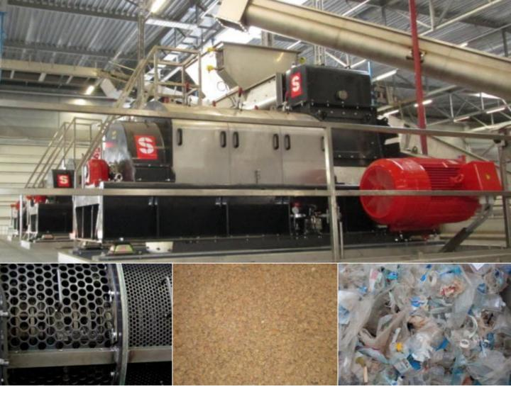
The SMIMO120 is suitable for processing and upgrading organic by-products. Capacity up to 35m<sup>3</sup>/hr and high separation efficiency make this design of machine unique.
