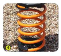
4- The springs are made from Grade 35SCD6 steel, shot blasted, stress relieved, zinc coated and finished with two coats of epoxy polyester powder.
