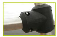
7- Injection moulded polyamide fixings connect the posts with the platforms and the various play features. They are non-toxic, flameproof and U.V. resistant. The thickness of the polyamide makes the equipement both strong and vandal resistant.
