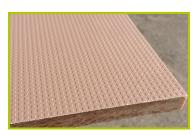
**3-** The platforms and the steps are made from a 12.5mm thick textured and non-slip compact material (HPL).
