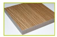
**3- The coloured panels** are made from a 13mm thick compact material (HPL). Robust in construction, it has excellent weather and vandal resistance properties.
