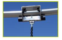
**12-The one-piece rail** is made of stainless steel,  $\varnothing$  76.1mm, 3.6mm thick. The trolley is made of stainless steel ensuring its durability.
