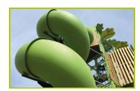
9- The slides are made of rotomouled polyethylene.
