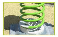
4- The springs are made from Grade 35SCD6 steel, shot blasted, stress relieved, zinc coated and finished with two coats of epoxy polyester powder. Proludic have patented an exceptionally strong and secure polyamide fixing for the spring, ensuring a long product life.
