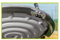
2- The pod seat is grey in colour and made from a single piece of rotomoulded polyethylene.It is fixed to a stainless steel frame that is fitted with buffers. The pod is suspended from swing chains covered with thermal retracted polyethylene.
