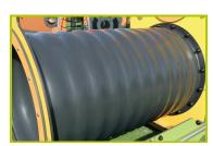
5- The tunnel is made of rotomolded polyethylene, 76cm in diameter.
