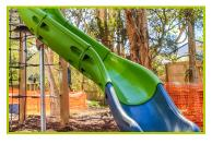
13-The Kayak slide is made of rotomoulded polyethylene.
