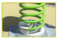
5- The springs are made from Grade 35SCD6 steel, shot blasted, stress relieved, zinc coated and finished with two coats of epoxy polyester powder. Proludic have patented an exceptionally strong and secure polyamide fixing for the spring, ensuring a long product life.
