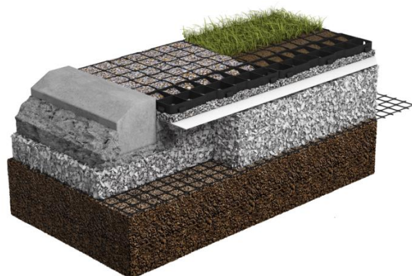
ABG Sudspave 40 permeable paver with Terrex NW9 separation geotextile
