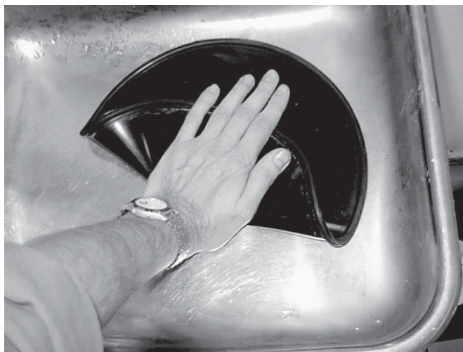
Figure 32 Washing technique of the membrane. Washing is done under water
