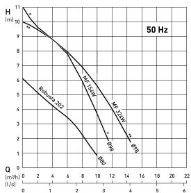
H = Total Head; Q = Discharge Volume Curves to ISO 9906 [60 Hz available on request]
