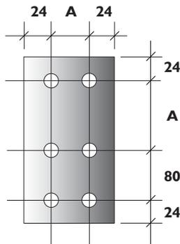
Galv steel 3mm thick 14mm dia holes
