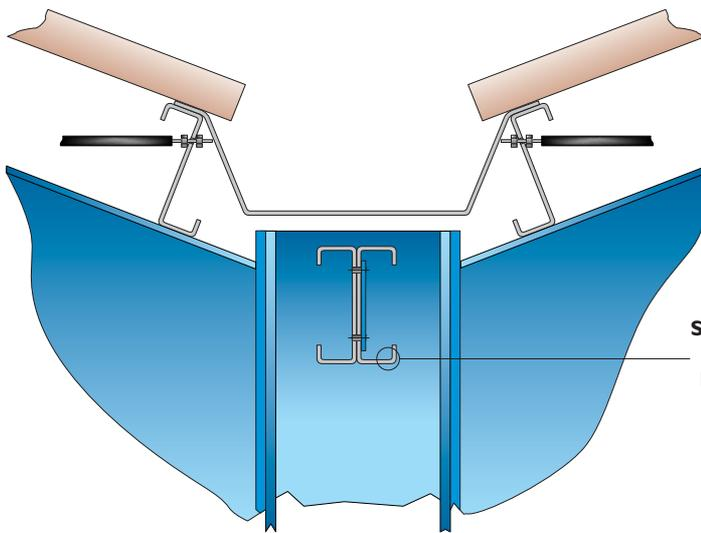
**HEAD TIE DETAIL WITH NO GUTTER SUPPORT**
