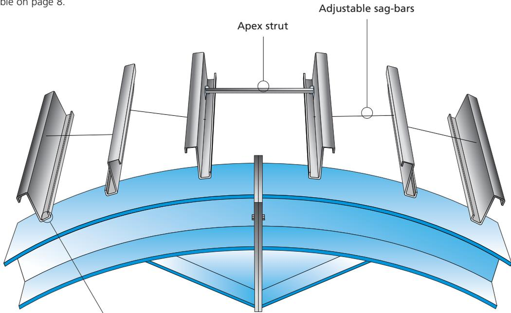
Alternative purlin directions reversed when roof tangent is less than 3°
