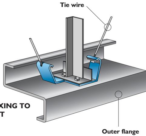
**DIAGONAL TIE FIXING TO RAIL STRUT**
