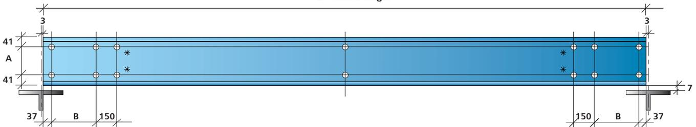
Sag bar holing at midspan for single row, at 1/3 spans for double row. 1/4 span for triple row.
