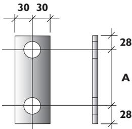
Galv 6mm thick plate 28mm dia holes
