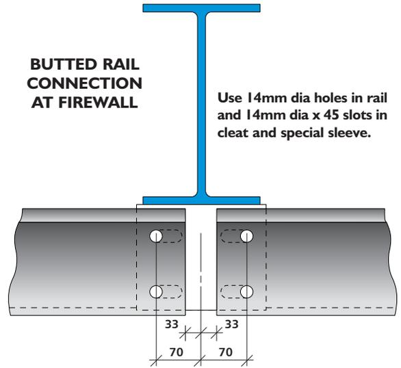
SEE DETAILING SECTION FOR DETAILS OF SPECIAL SUPPORT CLEAT
