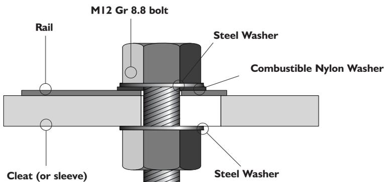
ENLARGED BOLT DETAIL SHOWING COMBUSTIBLE PLASTIC WASHER
