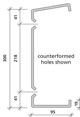
Rake to flanges available from 0 degrees to 35 degrees (above 35 degrees contact Steadmans)
