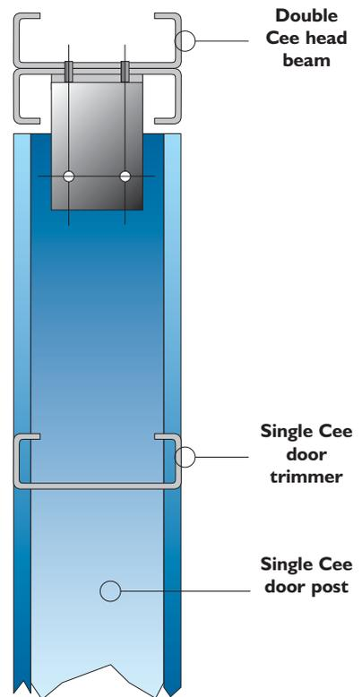
SECTION THROUGH TYPICAL OVERHEAD DOOR
