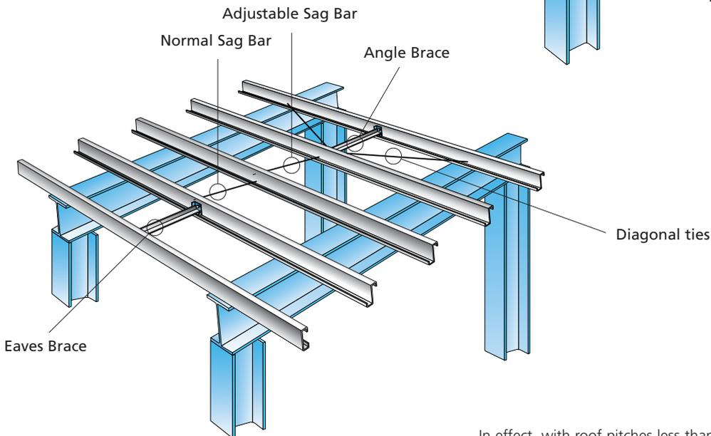
**PLAN ON ROOF WITH PITCH GREATER THAN 6°**
