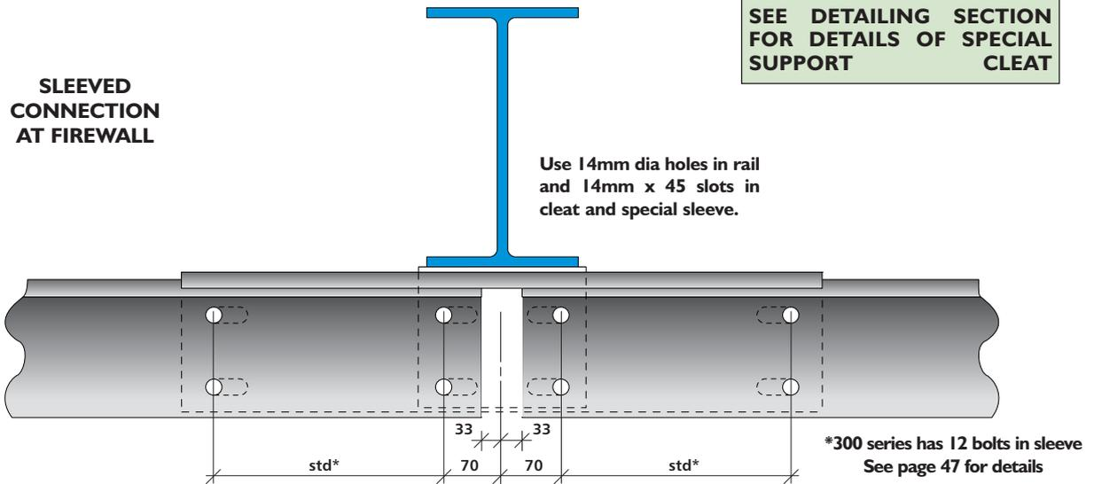
Details are shown here for zed rails but they apply equally to Cee section rails. See page 47 for detailing information.
