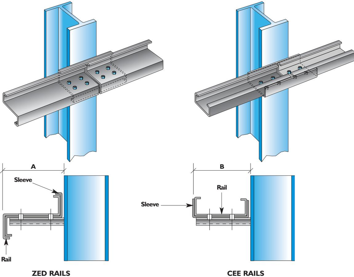
**ZED RAIL FLANGE TO THE CLADDING MUST TOE UPHILL FOR FIBRE-CEMENT, HOOK BOLT FIXED**
