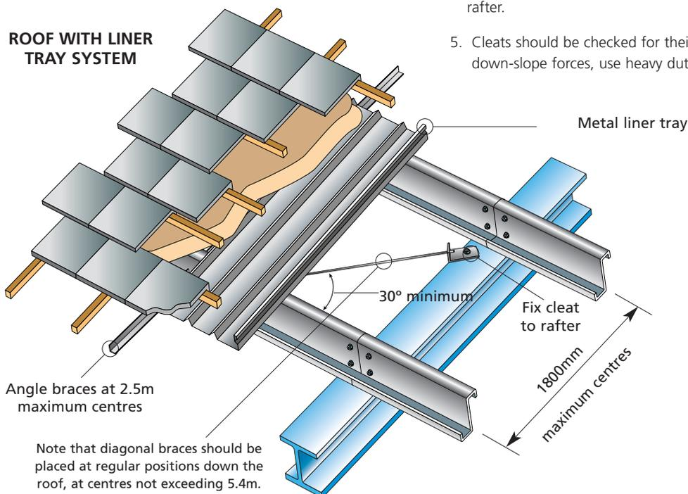
Note that diagonal braces should be placed at regular positions down the roof, at centres not exceeding 5.4m.
