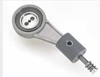
Piston – connecting rod subassemblies. Ready to install subassemblies with special roller bearings and large teflon base for guidance piston. Lightly built of aluminium. Replaceable with a few hand grips.
