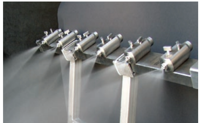
PCA spraying pattern with pressure nozzles
