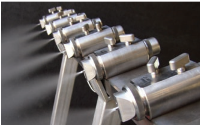
PCA spraying pattern with two-substance nozzles
