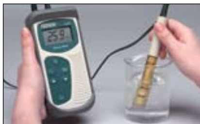
SALT 6 (35606-20) is ideal for measuring brines and aquaculture systems.
