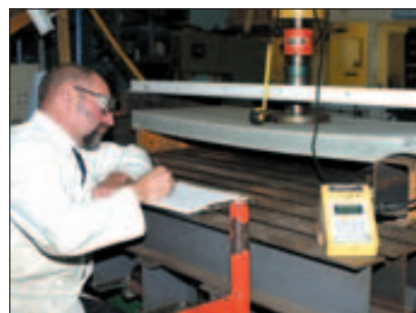
Dura Slab undergoing BS EN 124 testing
