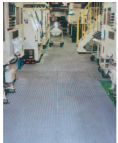
Fibreglass Grating anti-slip work area at car manufacturing plant
