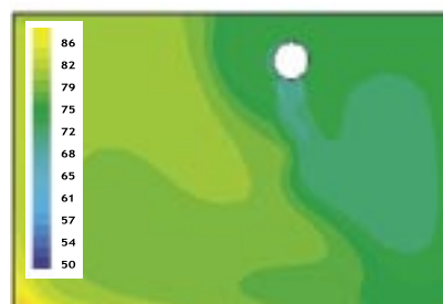
CFD graphic showing temperature gradient [°F]. Showing one fabric duct in exhibition hall.
