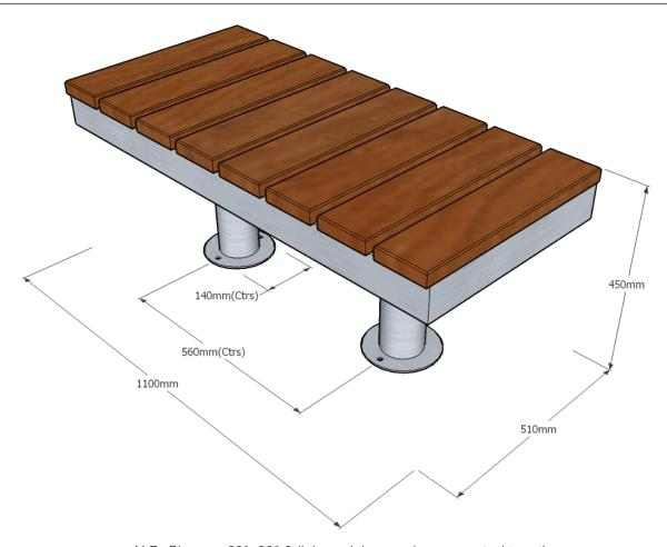
N.B. Chronos 69°, 90° & link modules can be connected together using special fixing brackets to create larger bench areas
