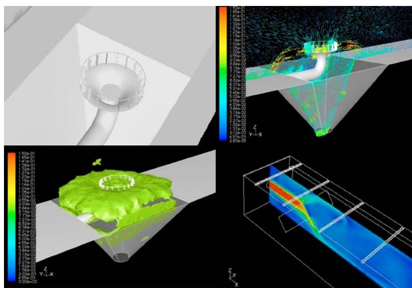
Improvements to the clarifier inlet were identified which could dramatically enhance the performance of the plant at high flows.
