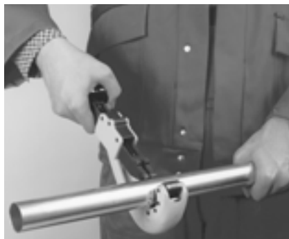
Figure 8.0-34 Cutting to length with pipe cutter
