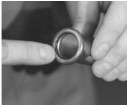
Figure 8.0-47 Checking seal ring
