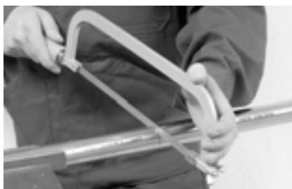
Figure 10.0-4 Cutting to length with fine-toothed hacksaw
