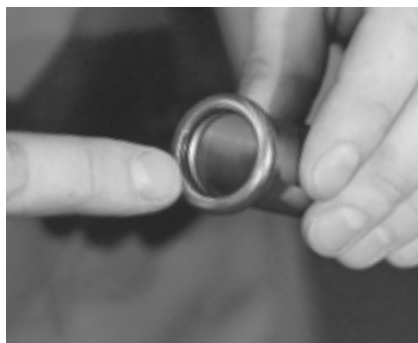
Figure 8.0-39 Checking seal ring
