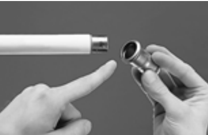
Figure 8.0-31 Checking seal ring
