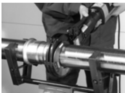
Figure 8.0-51 Pressing (ODs from 42 to 108mm)
