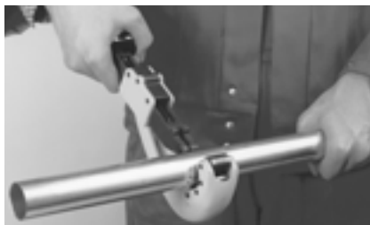
Figure 10.0-5 Cutting to length with pipe cutter
