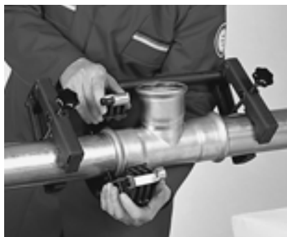
Figure 8.0-14 Putting pressing collar on
