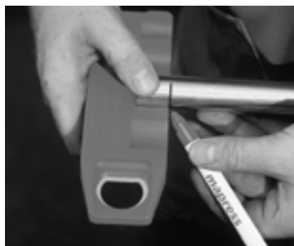
Figure 8.0-37 Marking insertion distance
