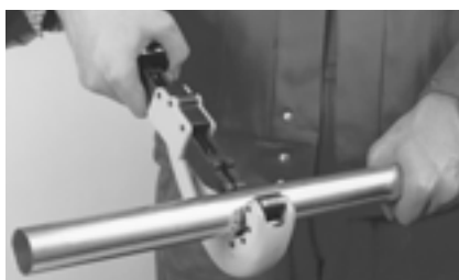
Figure 8.0-2 Cutting to length with pipe cutter
