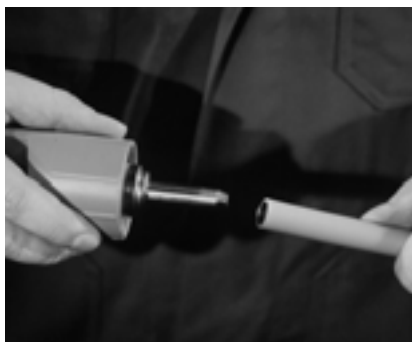
Figure 8.0-18 Using stripping tool to introduce sizing mandrel
