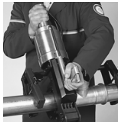
Figure 8.0-54 Pressing (ODs from 76.1 to 108mm)
