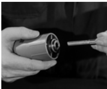
Figure 8.0-17 Stripping tool and calibrating mandrel
