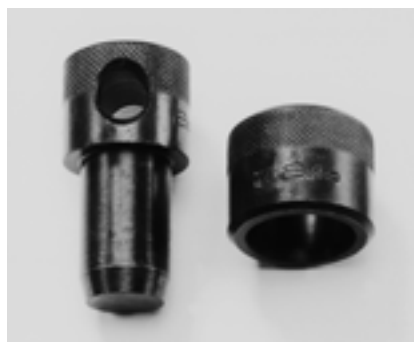
Figure 8.0-36 Sizing ring and sizing mandrel
