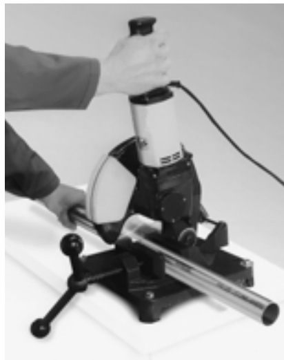
Figure 10.0-6 Cutting to length with electric saw
