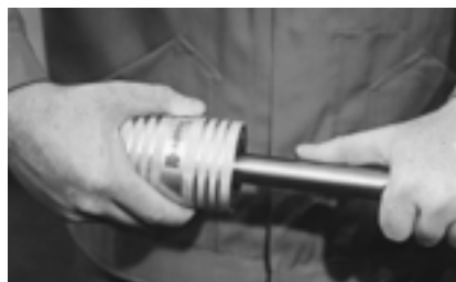
Figure 8.0-5 External deburring with hand deburrer
