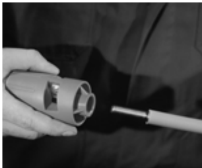
Figure 8.0-19 EDELFLX pipe with sizing mandrel driven in (plastic coating yet to be removed)
