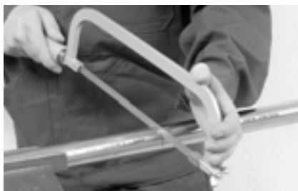
Figure 8.0-1 Cutting to length with fine-toothed hacksaw
