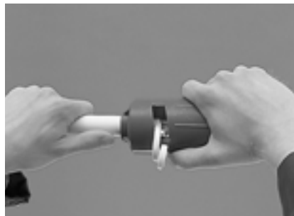
Figure 8.0-27 Stripping the plastic coating over the insertion distance
