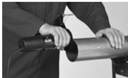
Figure 8.0-6 External deburring with RE1 electric pipe deburrer
