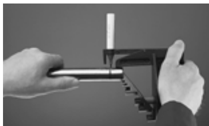
Figure 10.0-10 Marking insertion distance
