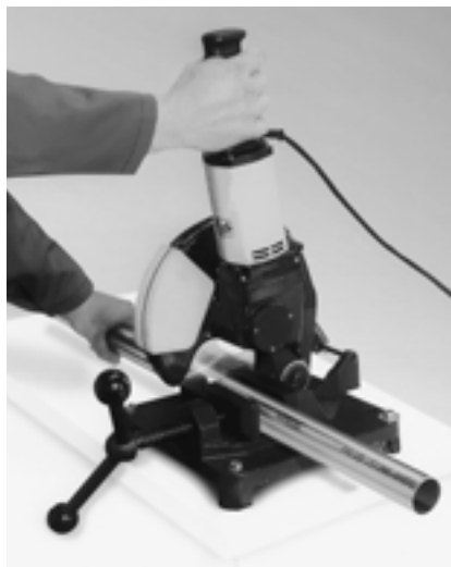
Figure 8.0-3 Cutting to length with electric saw
