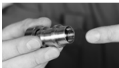
Figure 10.0-12 Checking sealing surfaces
