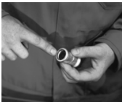
Figure 8.0-10 Checking seal ring
