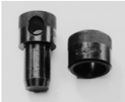
Figure 8.0-46 Sizing ring and sizing mandrel
