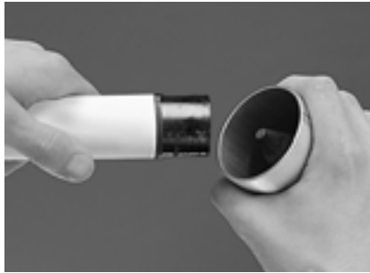
Figure 8.0-45 External and internal deburring with hand deburrer
