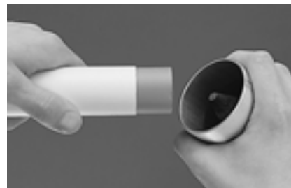
Figure 8.0-30 External and internal deburring with hand deburrer
