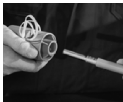
Figure 8.0-20 Stripping plastic coating over insertion distance
