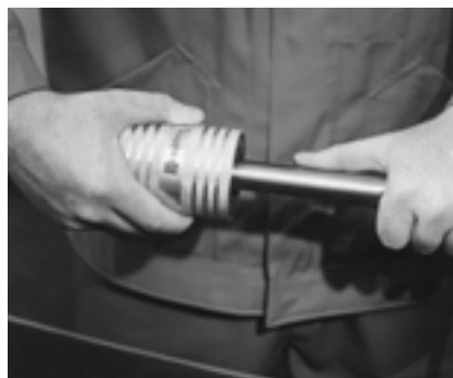
Figure 8.0-35 External deburring with hand deburrer
