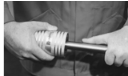
Figure 10.0-7 External deburring with hand deburrer
