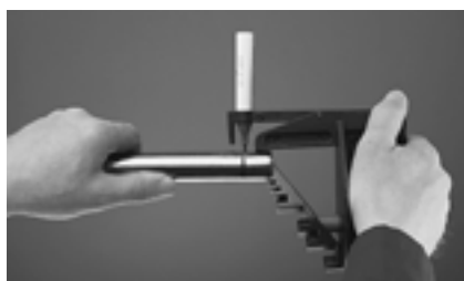
Figure 8.0-8 Marking insertion distance
