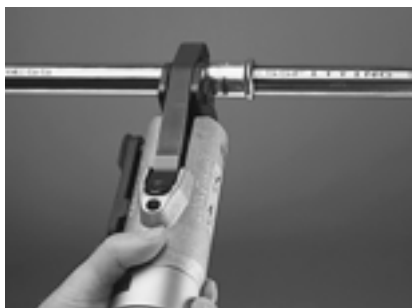
Figure 8.0-50 Pressing (ODs from 12 to 35mm)
