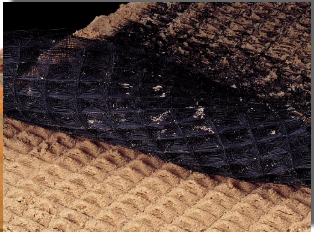
Demonstration of soil containment and interlock by pyramidal cells and ribs.
