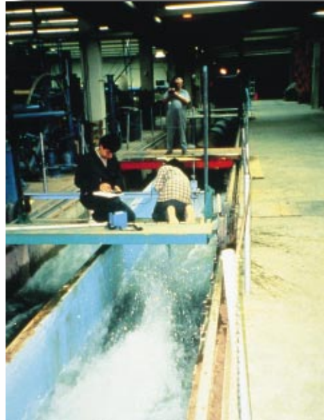
High velocity hydraulic flume testing.
