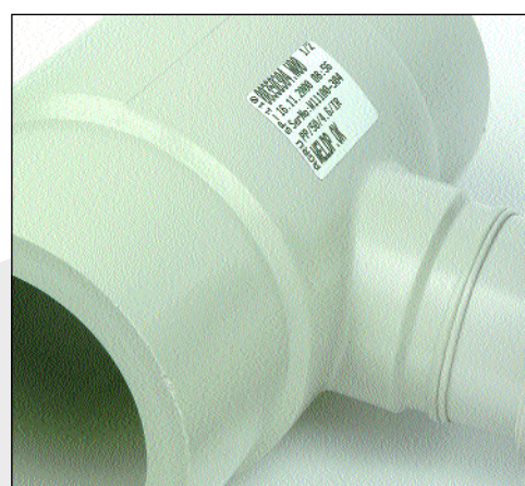
Completed IR weld and printed label
