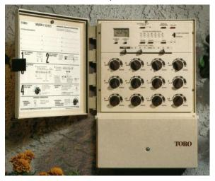
A standard irrigation control system comprises low voltage solenoid operated valves installed on each section of the garden or landscape, control cables laid from those valves, with the distribution pipework, back to the controller and the irrigation controller itself. The solenoid
