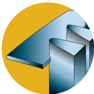
Each intersection of Vee-wire and support bar is welded to produce an extremely strong structure.
