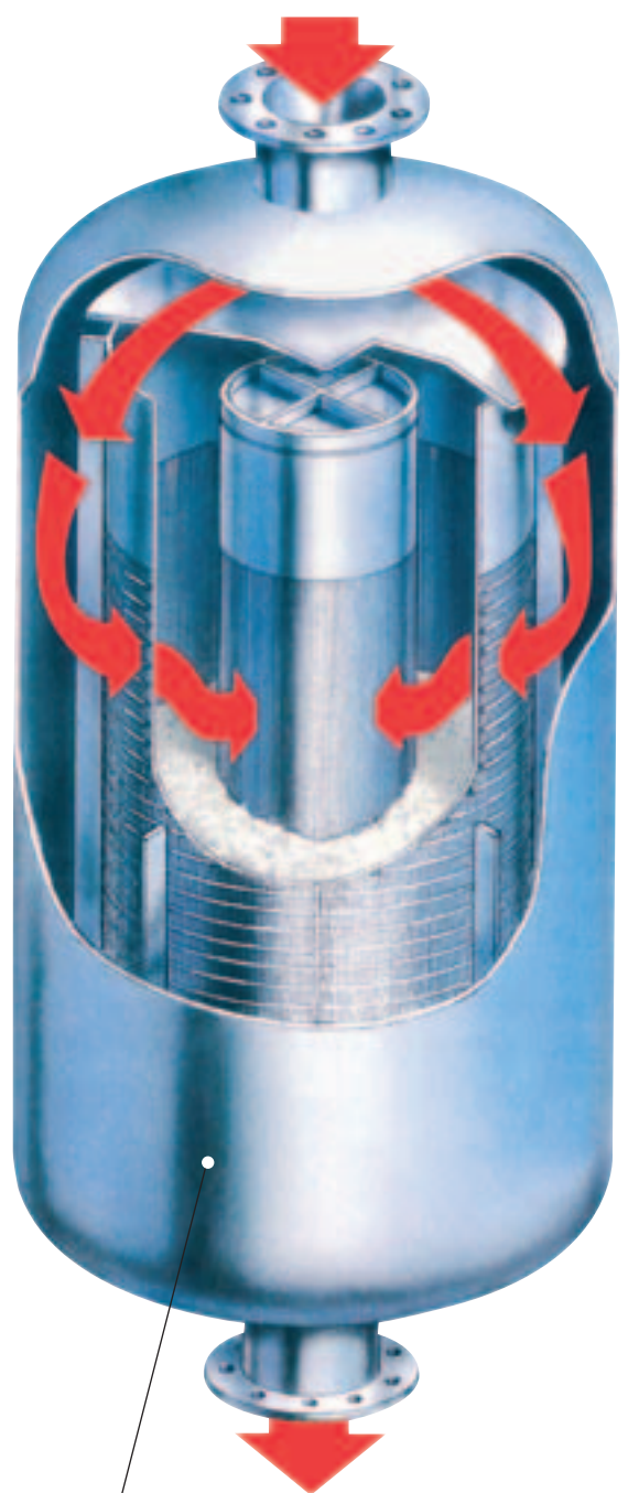
In downflow radial flow systems the process stream passes through the outer basket, across the catalyst and is collected in a center screen where it passes out the vessel bottom.
