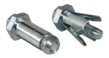
The complete fixing is inserted into a preformed hole in the spider or curtain wall brackets and ultimately into the main steel structure, the grade 8.8 bolt is then simply tightened to the recommended torque which in turn expands the fins of the main body to complete the connection.
