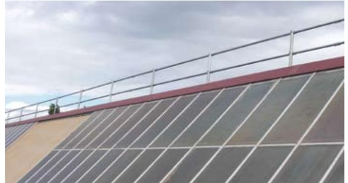
**KEEGUARD** Lite is supplied in prefabricated kit form, with the uprights, rails and fittings manufactured in Aluminium and grub screws supplied in Stainless Steel, and recycled PVC base weights. The lightweight system can be installed with minimal effort, thus saving time and money during on-site installation.
