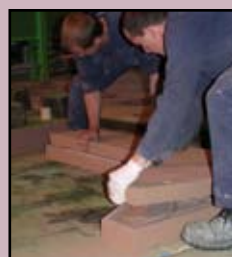
Joining the two halves of the mould prior to casting an architectural component.
