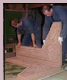
Joining the two halves of the mould prior to casting an architectural component.
