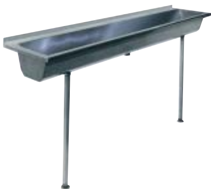
Olympic Washing Troughs Manufactured from 16swg 304 grade stainless steel with all exposed surfaces polished to a sateen finish. Supplied with stainless steel wall fixing brackets and C.P. waste outlet, diameter and position to suit client. Any required length up to 4800mm. Tap
