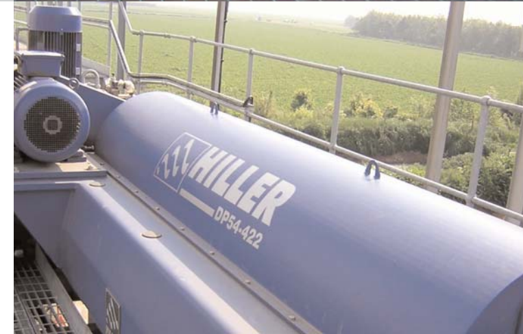
Centrifuge model DP54-422 potato factory effluent processing 40 m 3 /hr
