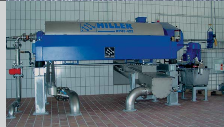
Centrifuge model DP45-422 dewatering 25 m 3 /hr of waste water
