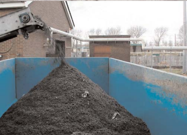
Dewatering of waste water treatment sludges.
