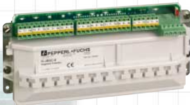
Segment Protector 8-spur DIN Rail mount Housing type: R
