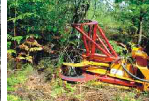
Felling head on 21 tonne excavator
