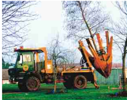
1.6m truck-mounted 4wd tree spade with flotation tyres
