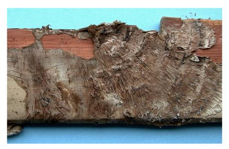
dry rot appears less likely as the result of 'capillary bound' moisture although once initiated such dampness will support growth.
