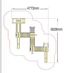
Wet Pour Safety Surfacing 0.6m FFH: 34m² x 20mm
