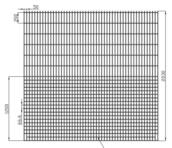
Each horizontal row consisting of two 8mm (Duo8) or 6mm (Duo6) wires, resistance welded at every intersection to 6mm verticals
